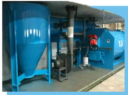
It is a dry filtration method. Located after the post-combustion, the cyclone retains the dust resulting from the incineration which is already oxidized in the post-combustion.
