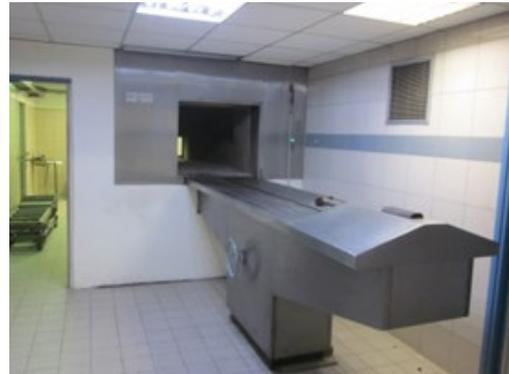
Its innovative and robust construction and its very dynamic design ensure a minimum of six cremations per 8 hours day. The cremation time is between 40 and 70 minutes and may be done without operator intervention. On-site installation, training and start-up are done by our teams.
