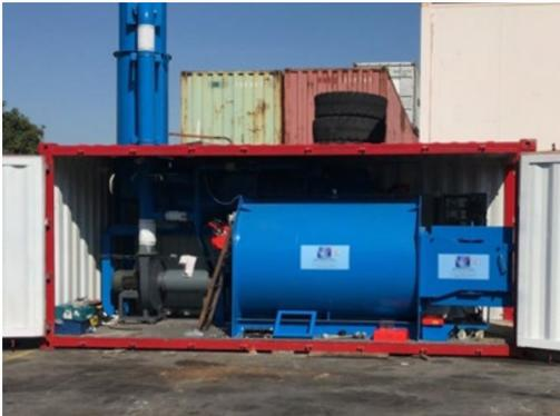
Embedded in a 20' container for mobility, this version allows transport and quick start-up on site. The pre-assembly is done in the workshop. The cremation time is between 40 and 70 minutes and may be done without operator intervention. On site, only start-up and heating are to be carried out.
